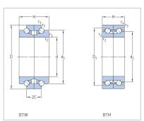
MONTON double direction angular contact thrust ball bearings are designed to in both directions. These bearings combination with locate spindle shafts cylindrical roller bearings in the NN 30 K or N 10 K series in the same housing bore. This bearing combination simplify machining of the housing bore.
